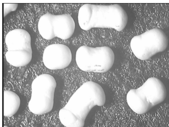
Figure 2. Stereomicroscopic image of dumbbell-shaped particles containing 60% theophylline (formulation 7 of theophylline) (8.5×).
